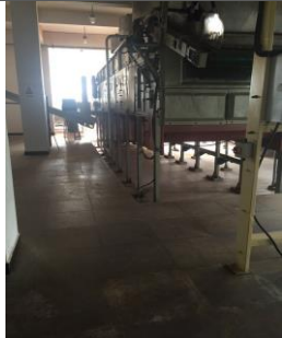
Photograph 4° yellow line has not been established yet around machineries with danger risk.
